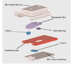
The Klixon® 7AM Thermal Protector is the market leader, backed by proven innovations in protection technology. The 7AM is a thermally operated snapaction device which delivers the maximum protection in the smallest package at an affordable price.
